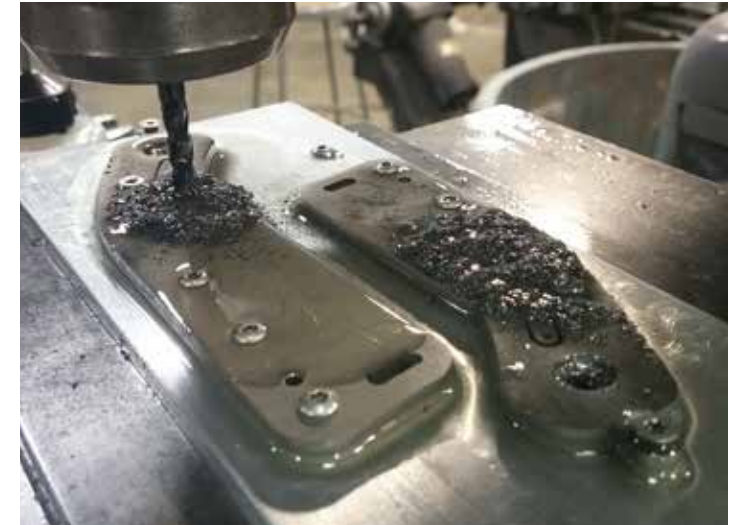
Counterboring titanium spring with 3/16 bit
