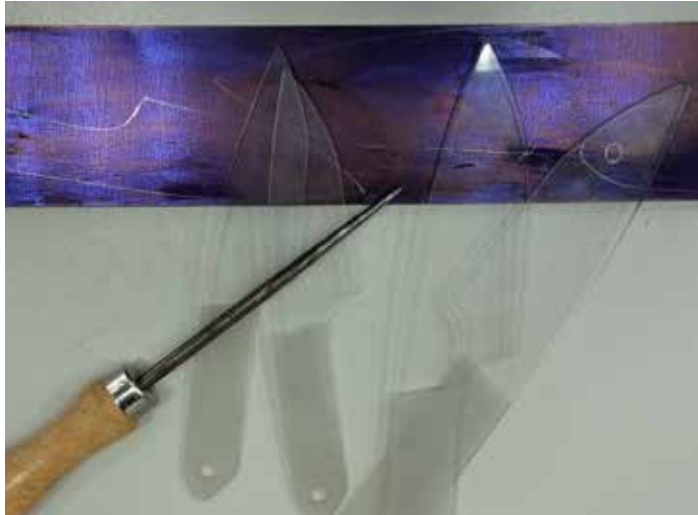
Laser cut templates used for scribing metal
