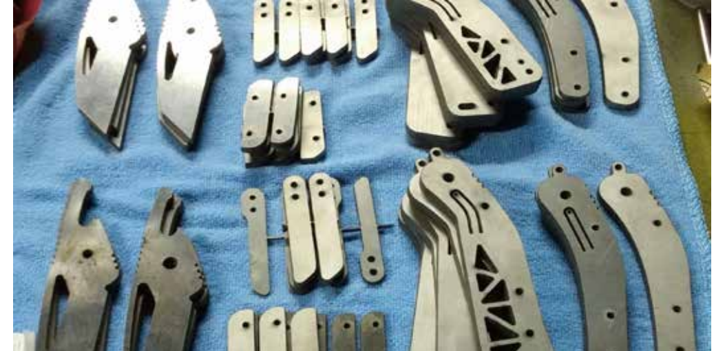
Parts made in .140 440C stainless, .160 and .060 Titanium
