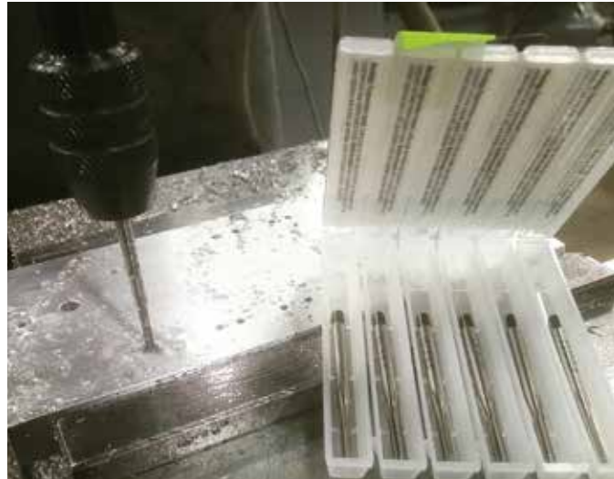
Hole pattern machined and tapped
