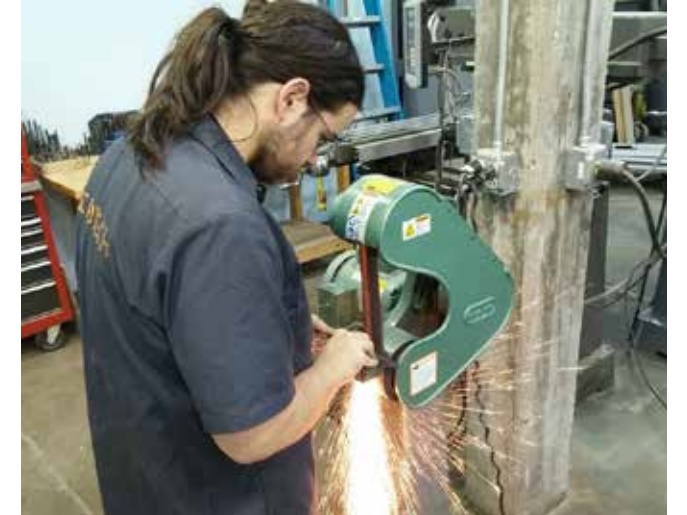
Profiles ground cleaning up dimensions
