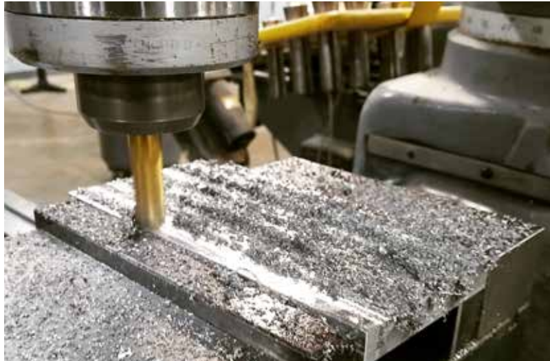
A .5 thick aluminum block machined square
