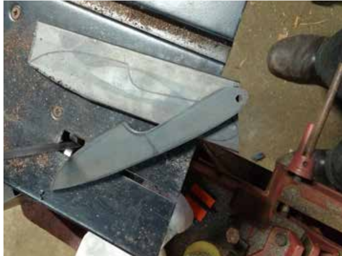
Practice blanks cut first using bandsaw
